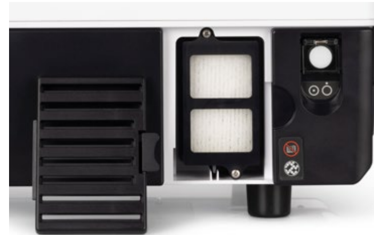
Dust Filter - clean/replace as needed. HEPA Filter – replace yearly
